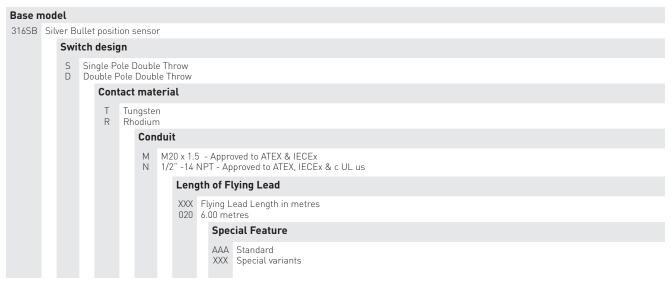
Example Code: 316SB-STM-020-AAA = 316 Silver Bullet, SPDT, Tungsten contacts, M20 conduit, 6 m flying lead & standard build.
