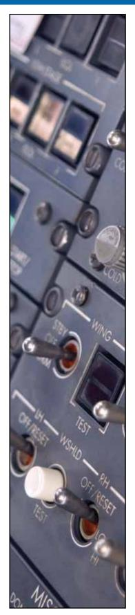
Hermetic and environmentally sealed toggle switches offer enhanced reliability with MICRO SWITCH™ technology. Can be used in a variety of applications where a panel-mount switch with an environment-proof rating is needed, including industrial equipment, military and commercial aviation, agriculture, process control, and medical.
